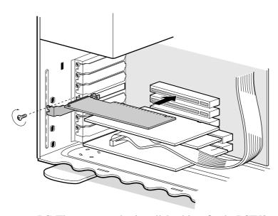
After installing it, start your PC. Then, you need to install the driver for the PCIU2.
